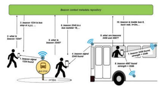
**Figure 26.** Mechanism to deploy connectivity between passenger device, roadside and on road infrastructure to manage service delivery, Juho Kostiainen, VTT Technical Research Centre of Finland (23rd World Congress, Scientific Session 12)
