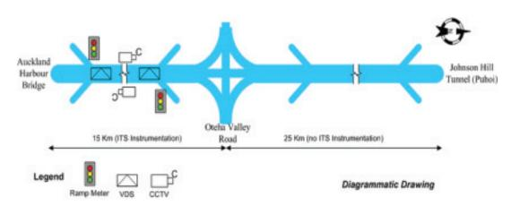
Figure 19. Schematic model of New Zealand managed motorway infrastructure with partial ITS instrumentation, Russell Pinchen New Zealand Transport Agency and Henry Wu JYW Consulting (23rd World Congress, Technical Session 33)
