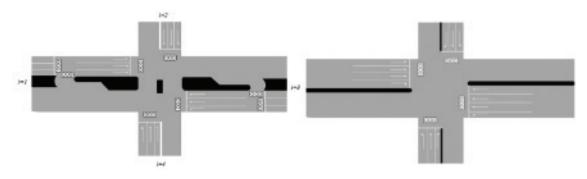
Figure 18. Non traditional approach to increasing intersection throughput requiring U turn to turn right (left diagram) instead of traditional design (right diagram). Note that no extra road space is required, Sandy Mae Gaspay, Institute of Industrial Science, University of Tokyo (23rd World Congress, Technical Session 4)
