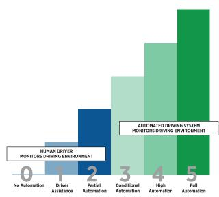
Figure 2. Levels of Driving Automation, Society of Automotive Engineers Australasia (SAE-A)^4  $\,$
